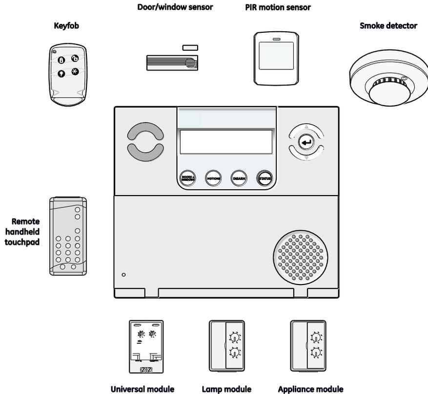
The security system uses sensors that communicate alarms to the control panel using radio waves.
