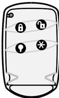
**Note:** For any key press on the keyfob, hold the button until the indicator light blinks.
